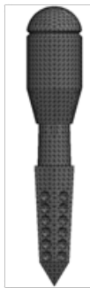
Figure 21: IHPP Implant Configuration 4 test with support – Mesh of the Mathematical Model with Tetrahedral Elements
